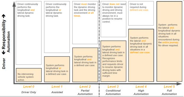
SAE L2 Definition: Driver needs to monitor → <sup>↓</sup> → SAE L3: Driver does not need to monitor
