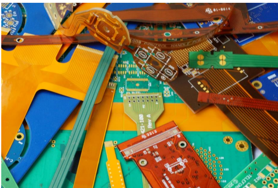
Fig. 1: Examples of various rigid, flex and rigid flex circuits illustrate the variety of choice
